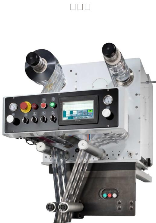
The Kurz Distorun machine module for processing single images and continuous designs by cold foil transfer
