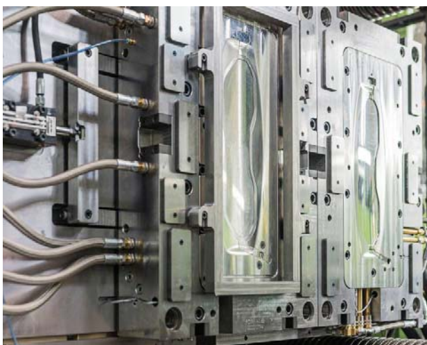
Injection mold for the IMD PUR process that is being shown at the Kurz booth (Photo: Kurz)
